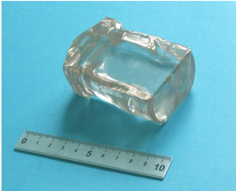
Figure 1: The crystalline boule of mixed (\text{Zn}_{0.9}\text{Cd}_{0.1})(\text{W}_{0.9}\text{Mo}_{0.1})\text{O}_4 crystal.
